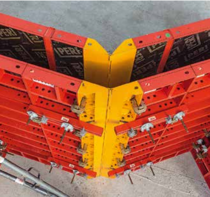
With the LIWA Articulated Corner, obtuse corners from 75° to 165° are formed; thereby compensation walers are to be mounted on the external corners.
