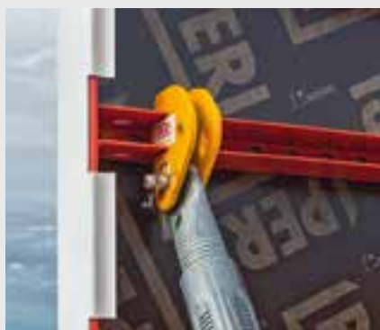
The simply designed LW Brace Connector for use on vertically-positioned panels can be attached to the anchor struts by means of bolts and cotter pins.
