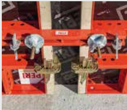
The compensation waler for compensations up to 25 cm with timber infill and filler plate.
